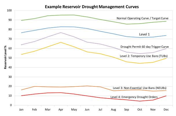
Figure 2.6: Example of reservoir control and trigger curves
