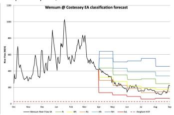
Figure 2.14: Example of Abstraction potential forecast and actual values completed at the start of the the summer (NH = Notably high, AN = Above normal, N = Normal, BN = Below normal, NL = Notably low and ExL = Exceptionally low)
