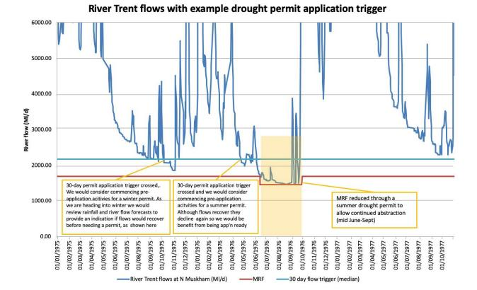
Figure 2.8: Worked example for River Trent direct intake showing drought permit trigger and activation
