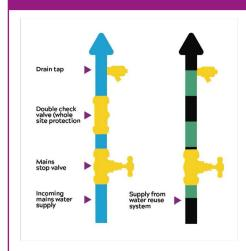
A double check valve must be installed immediately above the incoming stop valve at the point of entry.
