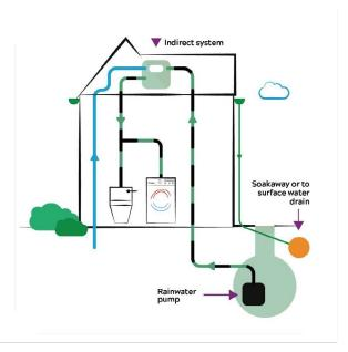
Water is pumped directly from storage such as an underground tank to the points of use such as a toilet.
