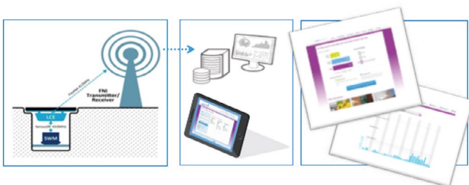
Figure 3.1: Data transmission from the customer to Anglian Water and back to the customer
