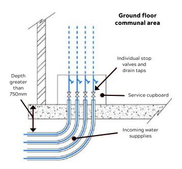
Figure 8: Showing typical arrangement separate incoming water supplies through with accessible cupboard to all occupiers.
