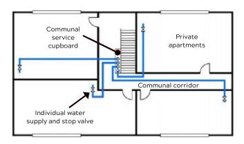
Figure 6: Routing of individual water supplies using communal areas.
