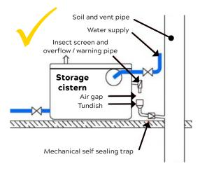
Figure 12: How to install an overflow discharging into a soil and vent pipe
