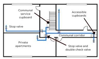
Figure 7: Pipe routing for a single common water supply to feed multiple apartments using communal areas.
