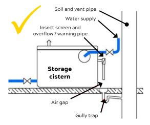
Figure 13: How to install an overflow using a gully trap
