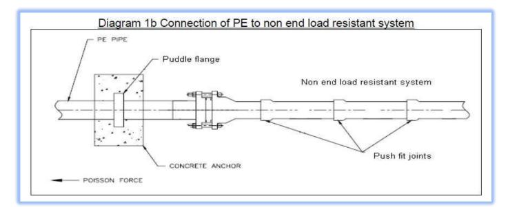
Consideration shall be given to using the pipe manufacturers design software / technical advice when designing the number, type and location of anchor points on ductile iron mains. This will enable the appropriate number of anchor points to be used and prevent over design.
