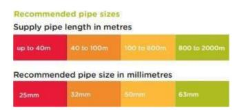
Services to multi-port manifolds shall be sized in accordance with the below table.
