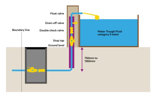
Stop-tap and double check valve in access chamber
