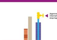
A BS 1010 internal stop tap must be installed as close as possible to where the pipework enters the property.
