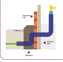
Your pipework enters the building at a depth of less than 750mm.
