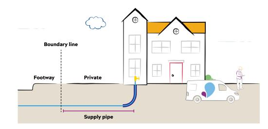
Ownership of a supply pipe depends on who is fed off that section of pipe, meaning some sections have joint ownership (sometimes known as common, shared or joint supplies). Since April 1990, the installation of common supplies is no longer accepted, meaning all new builds require an independent supply.
