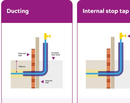
When the pipework enters the property it must be ducted in appropriately sized ducting.
