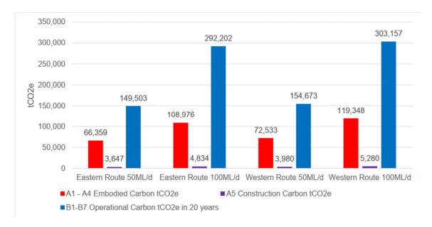
Figure 11-2: Whole life carbon estimates for Eastern and Western routes (both 50 ML/d and 100 ML/d capacities) (source: Arup)
