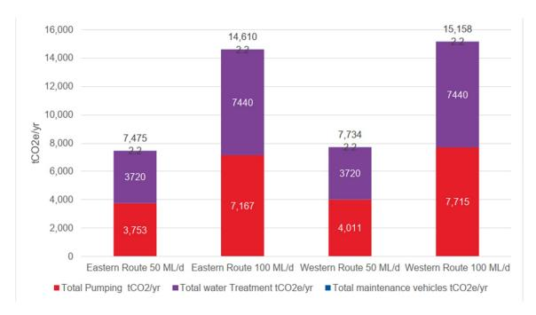
Figure 11-3: Operational carbon for Eastern and Western routes (both 50 ML/d and 100 ML/d capacities) (source: Arup)
