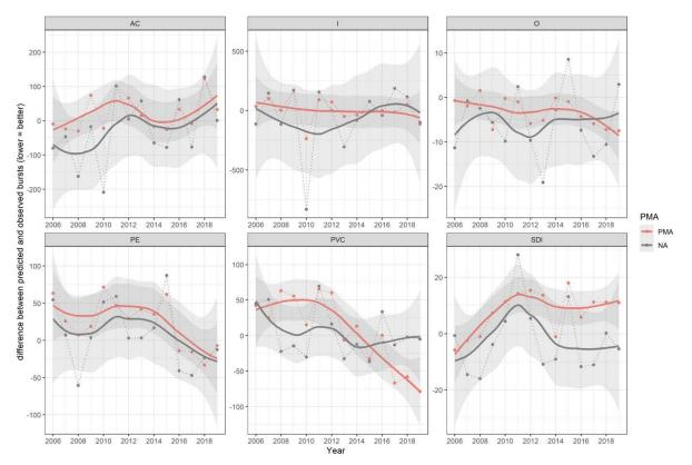
Figure 9: Observed bursts vs predicted bursts for Pressure Managed Areas (PMAs)
