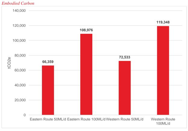
Figure 5. Embodied CO2e for Eastern and Western routes (50 Ml/d and 100 Ml/d)
