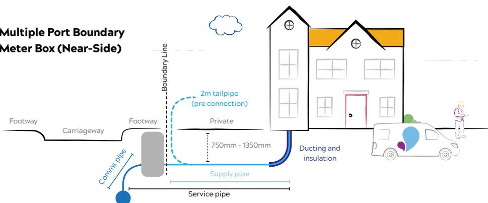
An alternative is available where the Developer can purchase and install the boundary box within the curtilage of the property, at the same time as they lay the supply pipe.
