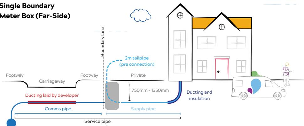
An appropriate location should be considered when installing supply pipes. If the chambers are positioned in a location which the Highway Authority do not deem acceptable, this can result in them refusing to adopt the road/footpath until they are repositioned. This work would be carried out at the Developer's cost.
