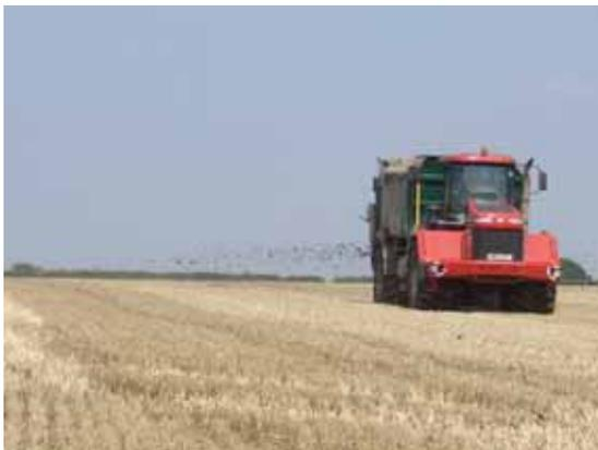
A tractor spreading treated biosolids, a by-product of the wastewater treatment process, to agricultural land as a high-quality soil conditioner.
