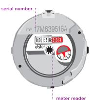
On the face of the meter, you'll see a series of eight digits. The first five white digits indicate cubic metres. The last three red digits are units of 10 litres.
