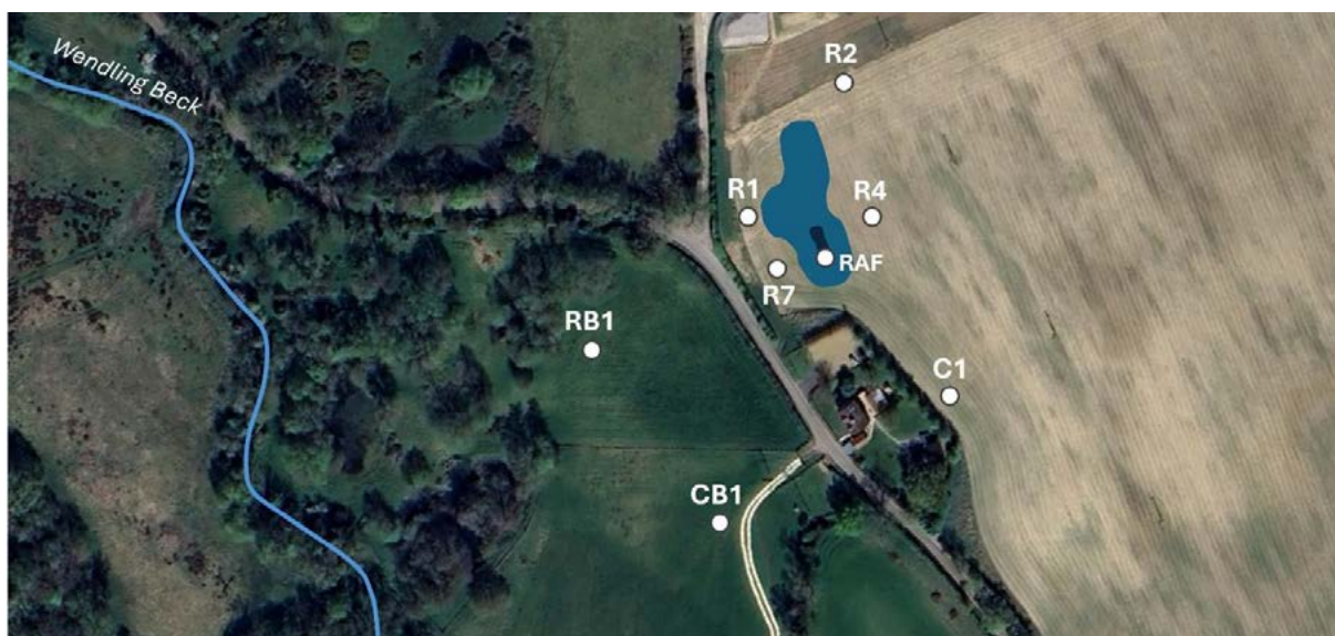
Figure 3- An example of a real life monitoring scenario of a RAF in the Wendling Beck. This demonstrates the Control-Impact monitoring approach whereby CB1 and C1 are the Control boreholes and the boreholes marked 'R' or 'RB' are the Impact boreholes. Source: WRE.
