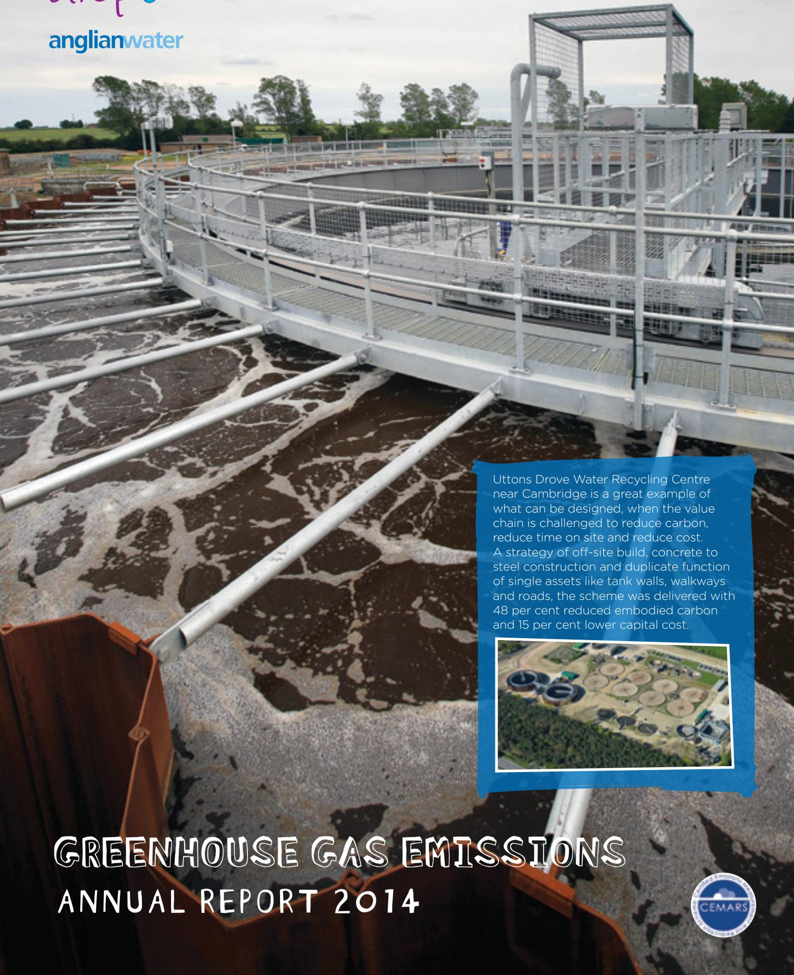
Uttons Drove Water Recycling Centre near Cambridge is a great example of what can be designed, when the value chain is challenged to reduce carbon, reduce time on site and reduce cost. A strategy of off-site build, concrete to steel construction and duplicate function of single assets like tank walls, walkways and roads, the scheme was delivered with 48 per cent reduced embodied carbon and 15 per cent lower capital cost.
